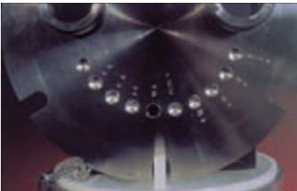
Picture 3 : Locating holes with locating pin
